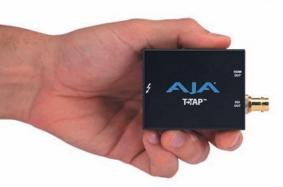
Small and simple to use, T-TAP connects direct to your Mac or Windows system via the blazing-fast Thunderbolt connection which provides the bandwidth necessary for full broadcast-quality video and audio output.
